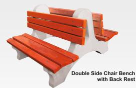
Each bench consists of 2 Nos base support in grey cement colour (Thickness:100mm, Back height:1000 mm & Front height:450mm, Base width:1435 mm) and 10 Nos. reinforced concrete planks in red colour of size 1500 X 100 X 50mm, and 2 No. of reinforced concrete plank of size 1500 X 200 X 50 mm (Planks can be in red color or Terrezzo finish)
