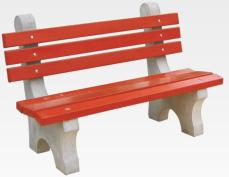
• Each bench consists of 2 Nos.L-shape base support in grey cement color (thickness:100 mm, Back height:1000 mm, front height:450 mm, Base width:620mm) and 5 Nos. reinforced concrete planks in red color of size 1500mm X 100mm X 50mm, and 1 No. of reinforced concrete plank of size 1500mm X 200mm X 50mm.
